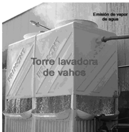
Fig. 8. Tower for direct washing of fumes.
